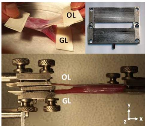
**FIGURE 3.** GL/OL compartment testing arrangement. A wider clamp was fabricated to span the entire tendon width. The specimen was aligned on the x-z plane. The abbreviations GL and OL indicate the points of force application that were coupled to these two layers; the cardboard marked OL was attached to connective tissue to which the OL fibers insert. The cardboard anchor on the OL's anchoring connective tissue was left long to avoid mechanical interference with the GL.
