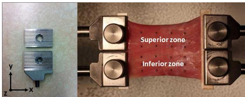
**FIGURE 2.** Transverse compartment testing configuration of medial rectus EOM. The specimen was aligned in the x-y plane. Metal bead fiducials are visible as an array of dots on the EOM global surface.
