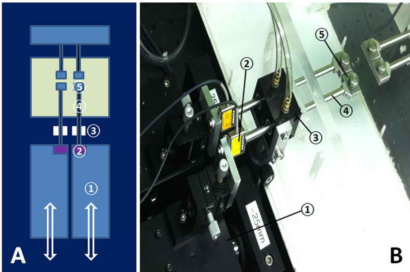
**FIGURE 1.** Dual channel microtensile load cell. **(A)** Schematic cartoon. Two linear motors moved independently, and generated tensile forces in each compartment of the tissue placed in the clamps. **(B)** Photograph of apparatus. In each adjacent channel, a linear motor (1) attached to a strain gauge (2) was coupled via a frictionless air bearing (3) through which passed a tensile shaft (4) connected to the specimen clamp (5).
