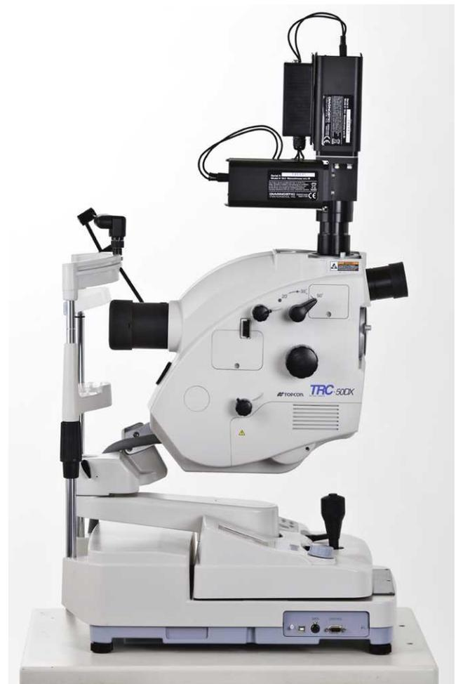
**FIGURE 1.** The dual wavelength retinal oximeter Oxymap T1 (Oxymap ehf.) is composed of two digital cameras (Insight IN1800, 1600 × 1200 square pixels; Diagnostic Instruments Inc.), a custom-made optical adapter, and an image splitter. It is coupled to a fundus camera base (Topcon TRC-50DX; Topcon Corporation).
