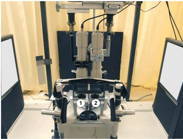
**FIGURE 1.** Picture of the experimental set-up. Through the use of two mirrors in the center of the set-up, each side screen presents the reading text to one eye only. The *small numbers* show the camera positions of the EyeLinkII system (1 and 2, one for each eye). These were positioned as close to the eye as possible to avoid reductions in measurement resolution and field view.
