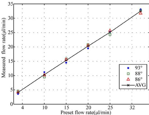
FIGURE 5. Calculation of the flow rate in a glass capillary filled with milk. The flow was controlled by a perfusion pump. The preset flow rates are  $32 \mu\text{L}/\text{min}$ ,  $25 \mu\text{L}/\text{min}$ ,  $20 \mu\text{L}/\text{min}$ ,  $15 \mu\text{L}/\text{min}$ ,  $10 \mu\text{L}/\text{min}$ , and  $4 \mu\text{L}/\text{min}$  at Doppler angles  $93^\circ$ ,  $88^\circ$ , and  $86^\circ$ .
