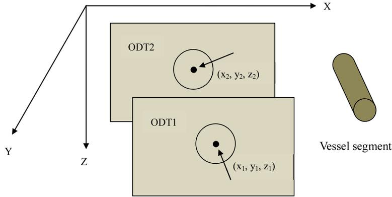
FIGURE 2. Illustration for Doppler angle calculation. A vessel segment appears on the two ODT images (ODT1 and ODT2) as a circular area. The centers of the circular areas have coordinates  $(x_1, y_1, z_1)$  and  $(x_2, y_2, z_2)$ . For a small segment the blood vessel can be treated as a straight line. The Doppler angle can be calculated from the two sets of coordinates.
