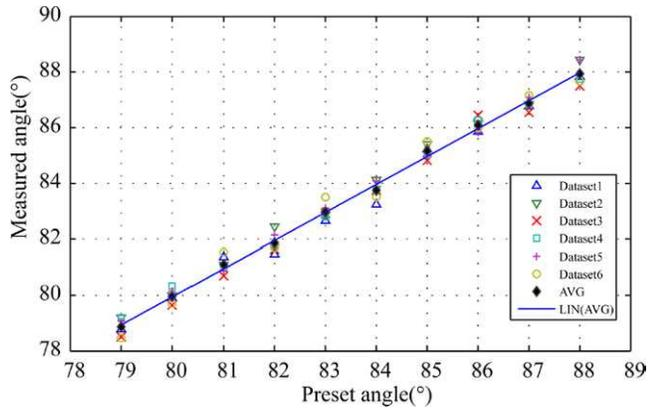
FIGURE 4. Validation of the angle calculation, using a flat plate as the sample.
