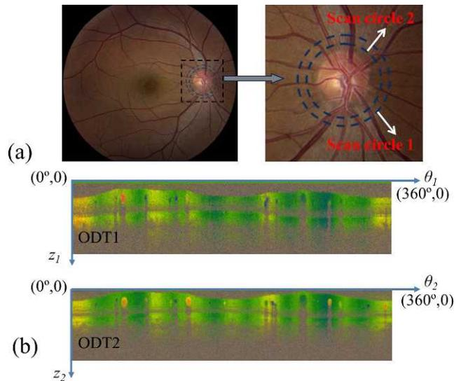
FIGURE 3. (a) Circular scan pattern centered on the optic disc in the dual-beam ODT system. (b) The ODT images simultaneously acquired by using the circular scan. The circular ODT images are displayed in the  $(\theta, z)$  plane, where the horizontal axis ( $\theta$ ) corresponds to the scanning angle from  $0^\circ$  to  $360^\circ$ ; the vertical axis ( $z$ ) corresponds to the depth dimension along the axis of beam propagation.
