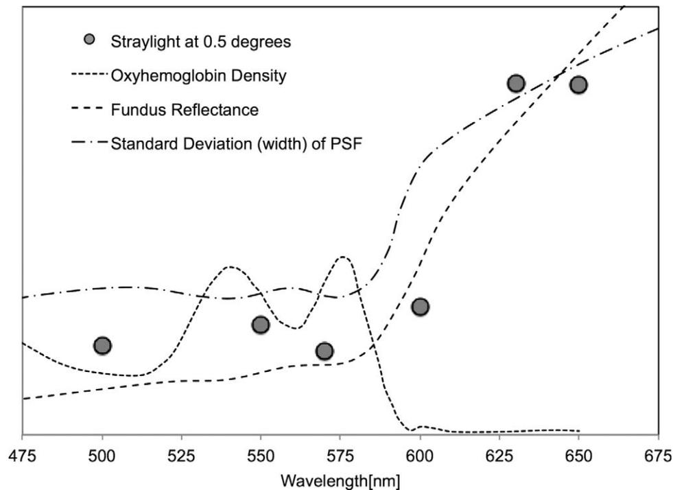
FIGURE 7. Straylight parameter at 0.5° (average of all subjects) and other spectral properties of the fundus. Oxyhemoglobin density is from Berendschot al.,<sup>21</sup> fundus reflectance from Delori and Pflibsen,<sup>22</sup> and the standard deviation (width) of the PSF from Hodgkinson et al.<sup>23</sup>
