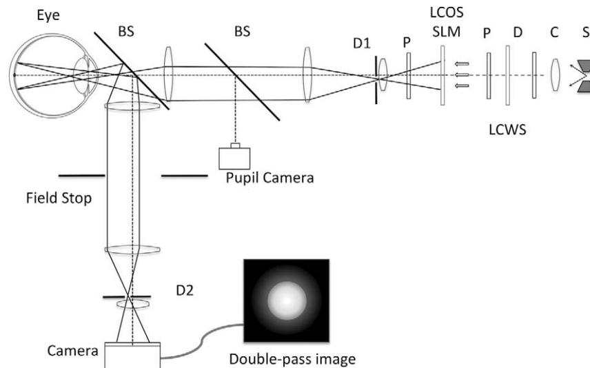
**FIGURE 1.** Schematic of the experimental system. S, xenon lamp; C, condenser lens; D, diffusers; P, linear polarizers; D1 and D2, diaphragms; LCWS, liquid crystal selectable bandwidth tunable optical filter; LC-SLM, liquid crystal modulator; BS, beam splitter.
