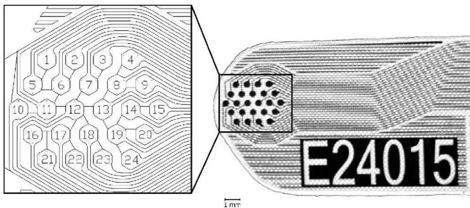
**FIGURE 2.** Photograph of actual 24-channel Pt electrode used in experiments (*right*) highlighting the number of each electrode (*left detail*). The electrodes are positioned to allow a hex guard configuration to improve charge containment. The form factor of the array is such that it is consistent with a planned 98-channel device undergoing development within the authors' labs.
