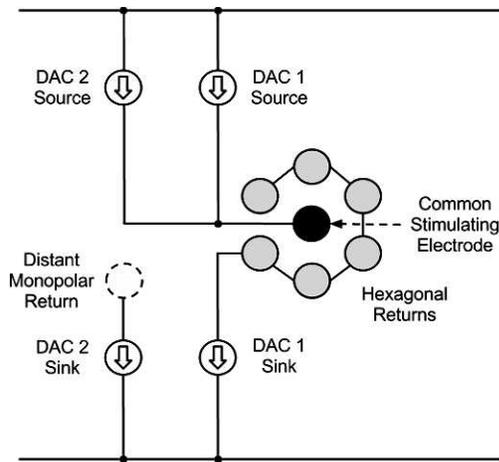
**FIGURE 1.** Quasimonopolar stimulation schematic. Two sources of the stimulator's constant-current DACs are connected to the same stimulating electrode (*black*), with the return paths of DAC1 going to the surrounding electrodes and the return of DAC2 going to a distant monopolar return.
