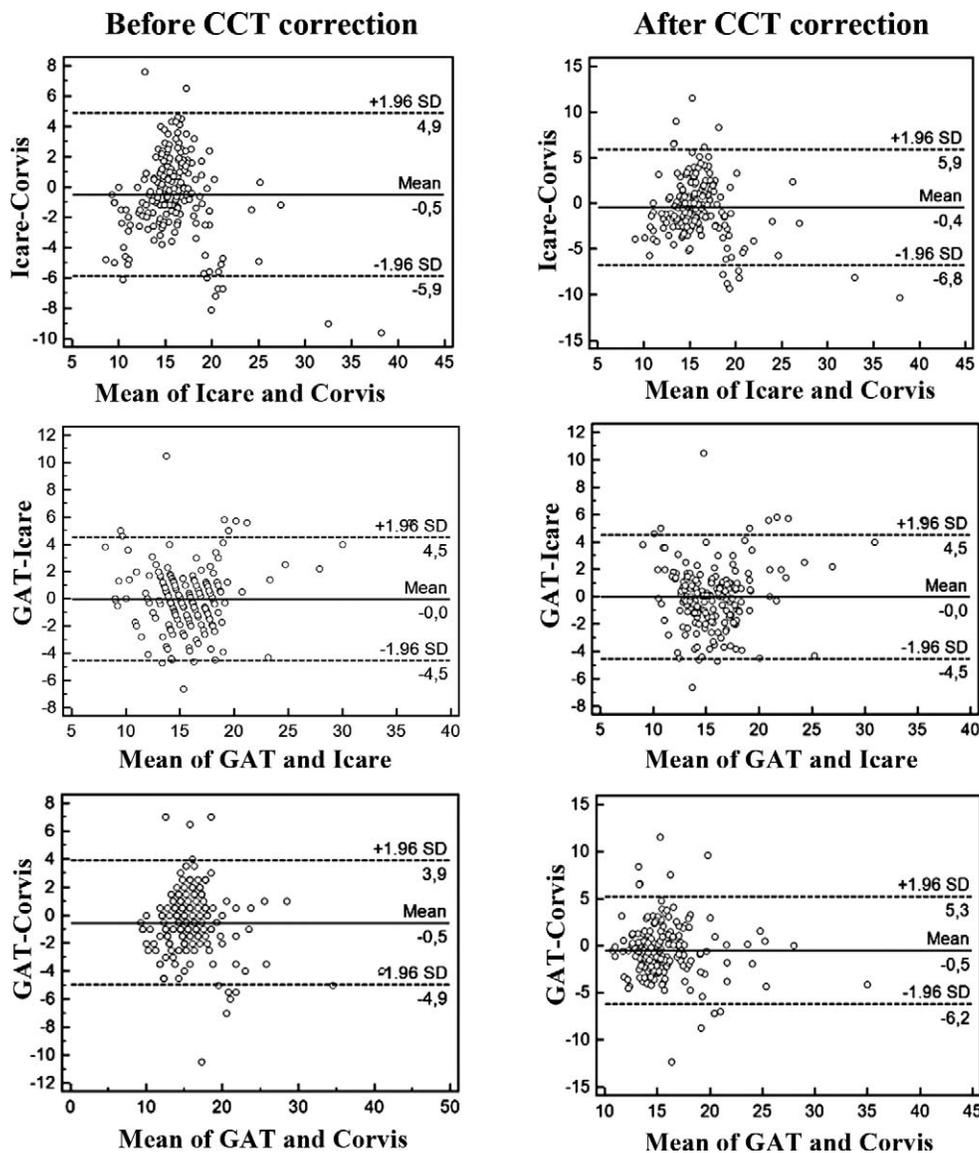
FIGURE 3. Bland-Altman plot of the agreement between the applied IOP measurement methods (before and after CCT correction). *Bold line*, the mean of the difference between these two methods; *dashed line*, 95% limits of agreement.
