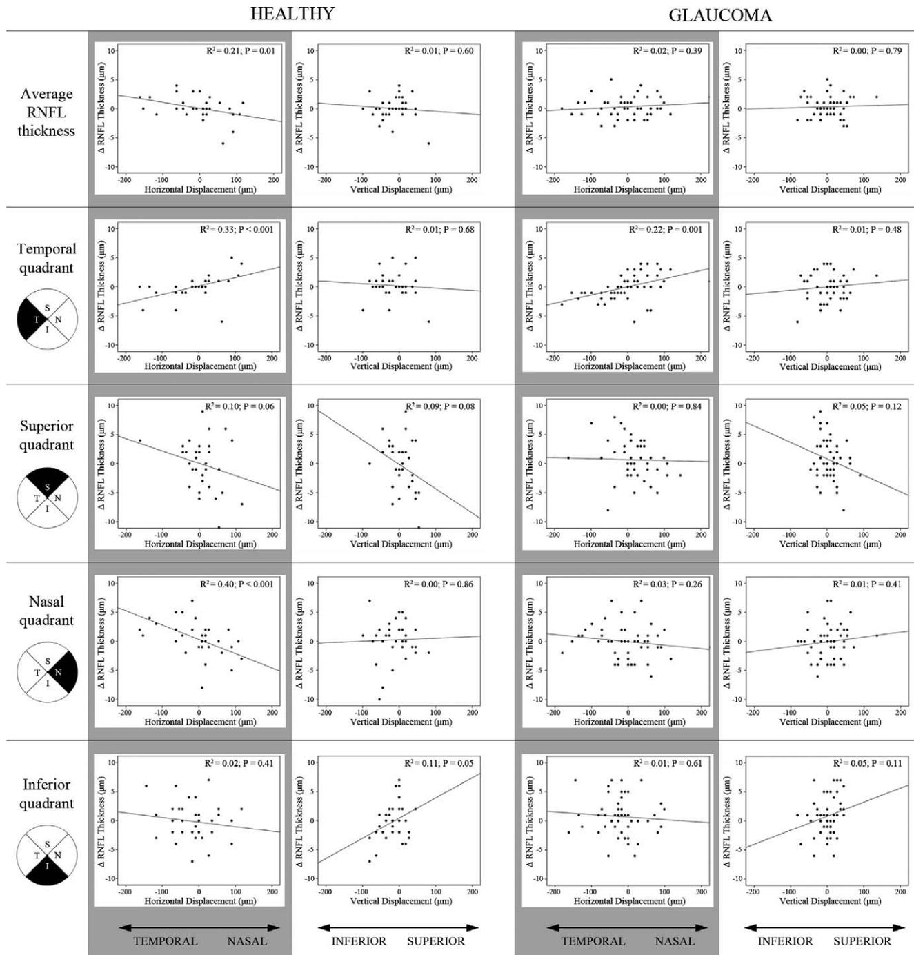
FIGURE 5. Regression plots of horizontal (grey background) and vertical (white background) scan circle displacement against change in RNFL thickness. Arrows (bottom) indicate the direction of the displacement.
