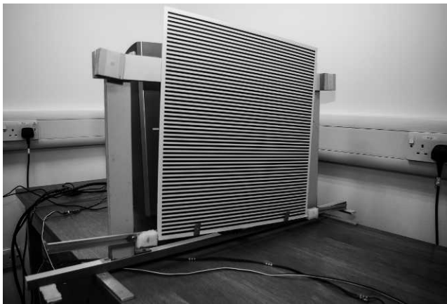
FIGURE 2. Computer-controlled platform used for automating grating orientation, shown here with the aperture removed.
