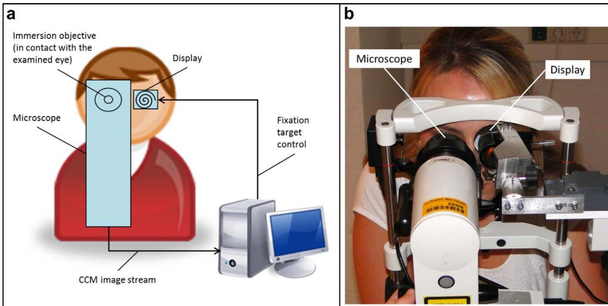
FIGURE 1. Corneal confocal microscopy examination setup with a small display arranged in front of the contralateral eye. (a) Schematic drawing and (b) experimental implementation.
