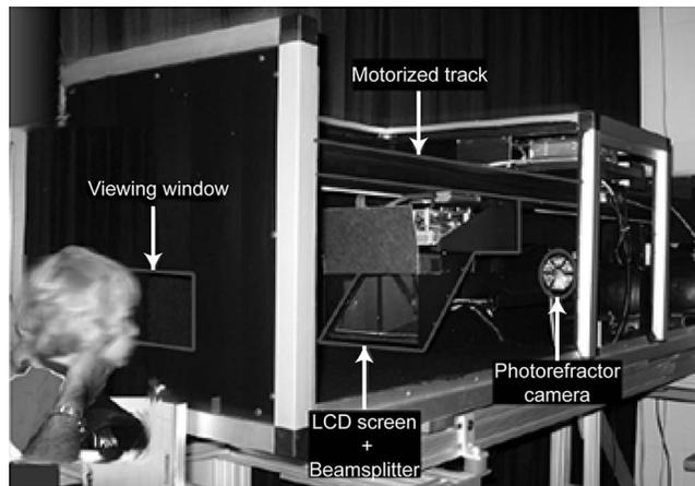
**FIGURE 1.** Experimental equipment. Subjects viewed a cartoon movie displayed on a horizontally mounted LCD screen via a beam splitter, while the PR camera (at 1 m) measured eye alignment and refraction. The LCD screen and the beam splitter were mounted on a motorized track and placed at a viewing distance between 33 and 90 cm depending on the condition.
