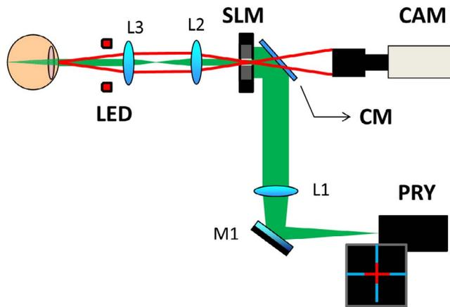
**FIGURE 1.** Schematic layout of the instrument. A pico-projector (PRY) produces a two-color stimulus that is seen through the small aperture created by the spatial light modulator (SLM). The corneal reflex produced by a semicircular array of LEDs is recorded by means of a camera (CAM) with a telecentric objective through a cold mirror (CM).
