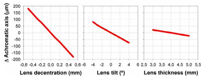
FIGURE 7. Changes in the position of the achromatic axis intersection with the pupil plane (AcP) as a function of lens decentration, lens tilt, and lens thickness.
