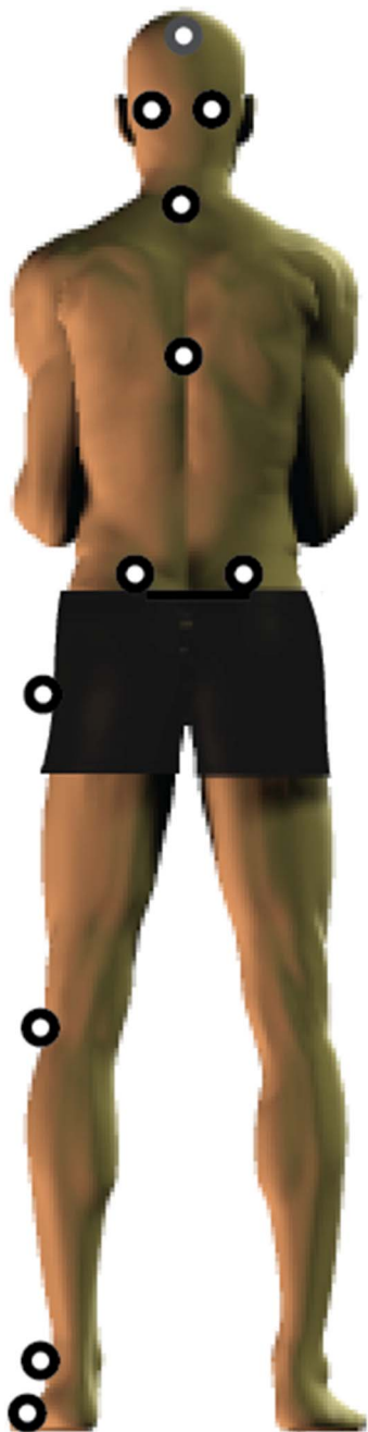
FIGURE 1. Graphic representing head and body locations of infrared markers used to record location and calculate joint angles and body segment orientations (see Methods for description). Note that due to camera location, leg markers were placed on the left side only. The front head marker was off-centered to the left . Gray color of one marker on the head indicates that this marker was on the front of the head.
