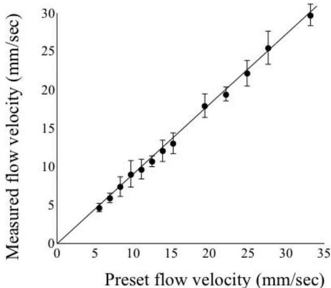
FIGURE 2. The relation between the preset flow rate and measured flow rate by segmental-scanning DOCT in vitro for three measurements in three glass capillaries. Data were expressed as the mean  $\pm$  SD ( $n = 3$ ). mm/sec, millimeters/second.
