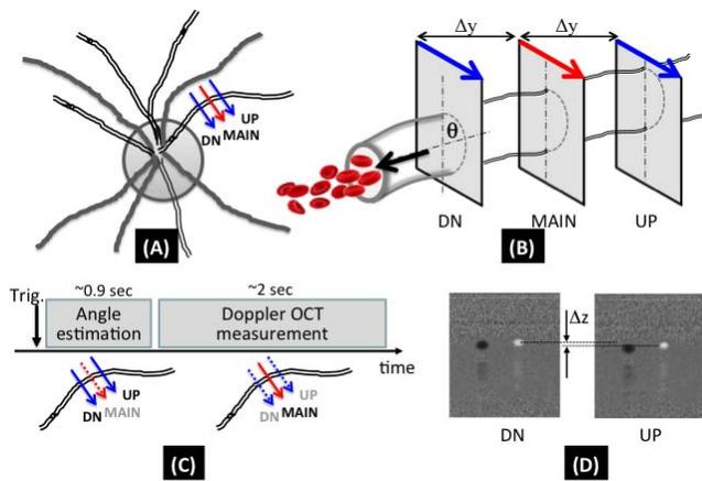
**FIGURE 1.** Illustration of a Doppler angle and velocity measurement using the segmental-scanning DOCT method. (A–C) The Doppler angle is measured with two alternative scans (UP and DN) in separation of  $2\Delta y$  followed by main scan (MAIN) for 2 seconds. (D) Using the phase image from two alternative scans (UP and DN), the centers of the vessels are identified to calculate the incident Doppler angle.
