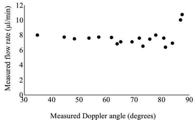
FIGURE 3. The flow rates measured with different preset Doppler angles. The Doppler angle is changed at the various angles of the glass capillary with constant preset flow. The measured flow rate seems stable under 85 degrees but is overestimated over 86 degrees of the Doppler angle measured by segmental-scanning DOCT.
