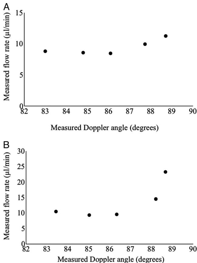
**FIGURE 5.** The measured flow rates at various Doppler angles by tilting the head of the cat. The measured flow rates in the arterioles (A) and venules (B) seem stable under 85 degrees but overestimated over 86 degrees of the Doppler angle measured by segmental-scanning DOCT.
