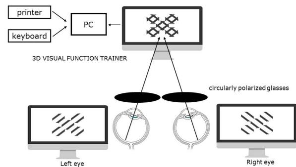
**FIGURE 1.** Dominance measuring system. All stimuli were generated on a 24-inch LCD monitor (P240W; Hyundai; pixel solution, 1980 × 1200) using VisageSage (3D Visual Function Trainer; Japan Focus Co., Ltd.).
