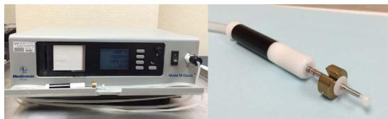
FIGURE 1. Pneumatometer and its probe, which has a flat tip with an external diameter of 5.3 mm. The weight on the probe is used only for tonography.
