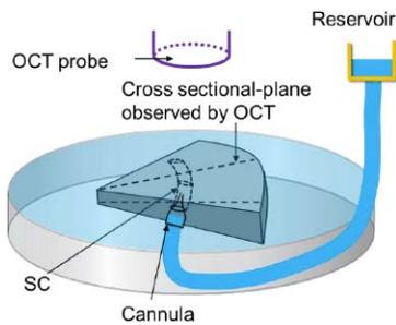
**FIGURE 1.** Schematic overview of experimental setup, including the SD-OCT system, a reservoir used for controlling pressure in SC, a cannula, and a Petri dish. The *triangular-shaped object* is a wedge of limbal tissue.
