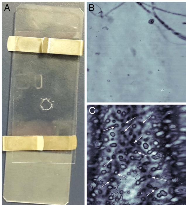
**FIGURE 2.** (A) Cornea tissue sample stabilized between a soda-lime substrate and a cover glass with 5-mm window for imaging and fixated. (B, C) Acoustic GHz-micrograph of 500  $\mu\text{m}^2$  size, recorded at 1 GHz with the acoustic lens focused on the top surface of the glass substrate for samples of normal cornea tissue (B) and cornea tissue with guttata (C). The *white arrows* in (C) indicate examples of guttata with the granular structures characteristic of guttata endothelia.
