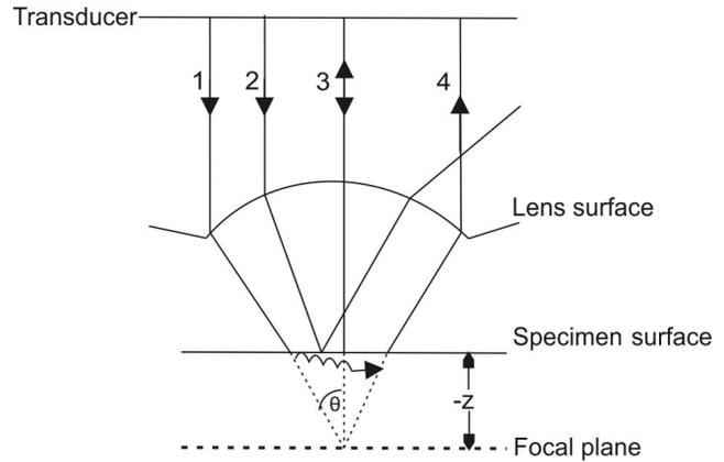
FIGURE 1. Illustration of the different rays that can contribute to the formation of the  $V(z)$  collected by a negatively defocused lens (defocusing toward the sample).
