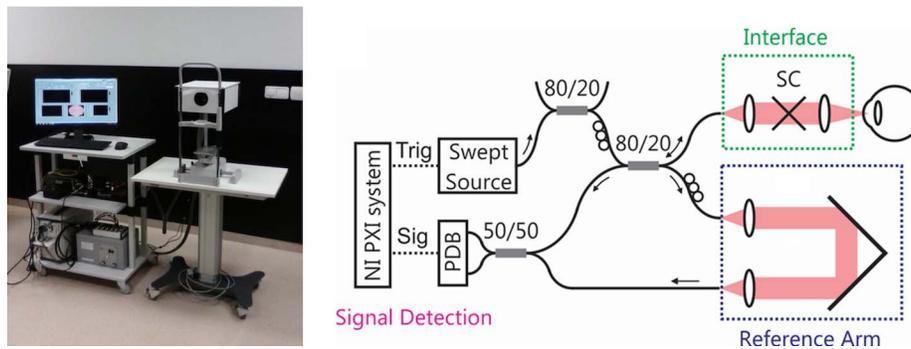
**FIGURE 1.** Photograph and scheme of the long-range SS-OCT setup at 1050 nm. A Thorlabs (Newton, NJ, USA) balanced photodetector (PDB) and a National Instruments (Austin, TX, USA) acquisition system (PXI) were used to detect and acquire the interferometric signal. Galvanometric scanners (SC) enabled lateral beam scanning of the eye.
