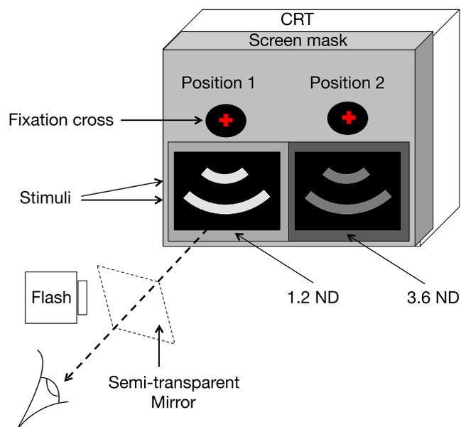
**FIGURE 1.** Experimental setup. Observers initially fixated the red cross at position 1. When sensitivity increased so that the intensity was below  $-2.5$  log Scotopic  $\text{cd}\cdot\text{m}^{-2}$ , the red fixation light and the stimuli moved to position 2. Before each experimental session the flash unit delivered a selective bleach to the area of the retina corresponding to the stimulus. The foveal region was not bleached.
