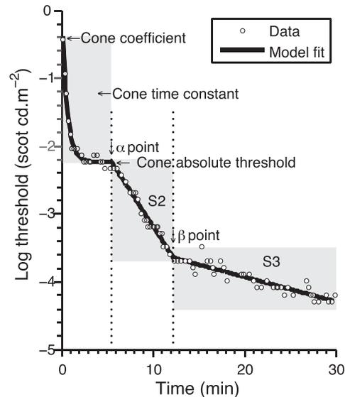
**FIGURE 2.** Typical DA curve for a young, healthy observer measured inferiorly at  $5.5^\circ$  eccentricity, following a bleach of 97%. Grayed areas show the cone-dominated recovery phase and the S2 and S3 phases.  $S2 = -0.26 \log_{10}$  scot  $\text{cd.m}^{-2}.\text{min}^{-1}$ ,  $\alpha = 5.39$  minutes and  $\beta = 12.24$  minutes.
