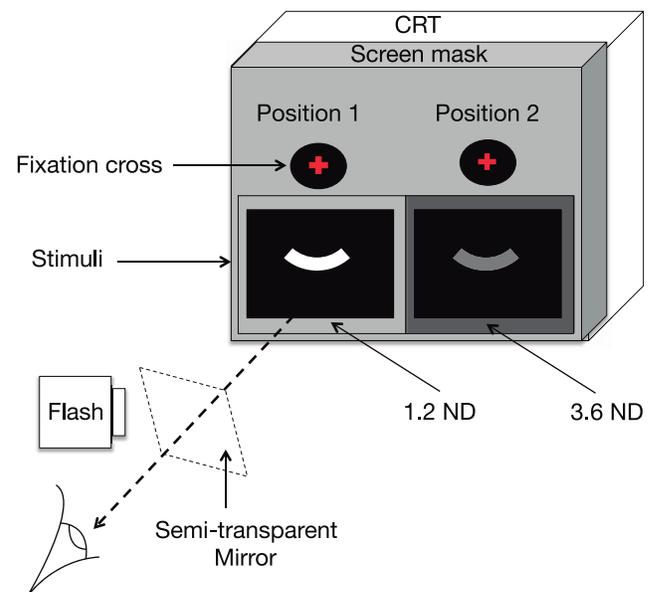
**FIGURE 1.** Experimental setup. When the threshold fell below  $-2.5 \log \text{ cd/m}^2$ , the fixation cross and the stimulus moved to position 2 where an additional 2.4  $\text{ND}$  filter was attached. This gave a total filtered luminance range of 6.5  $\log$  units ( $0.8$  to  $-5.7 \log \text{ cd/m}^2$ ). The location of the photobleach was controlled by aligning the flash with the stimulus (at position 1) through the semitransparent mirror.
