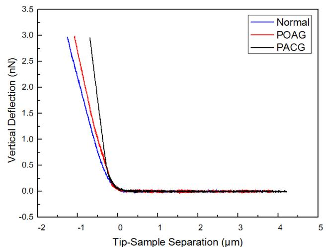
**FIGURE 3.** Representative force-distance curves showing different stiffnesses of the human irides.
