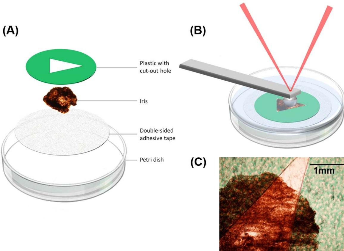
**FIGURE 1.** (A) Schematic diagram showing the iris sample mounted on a petri dish for AFM measurements. (B) AFM cantilever with a 4.5 μm diameter spherical bead was used for stiffness measurements. (C) Optical image of a mounted iris sample with the anterior surface exposed.
