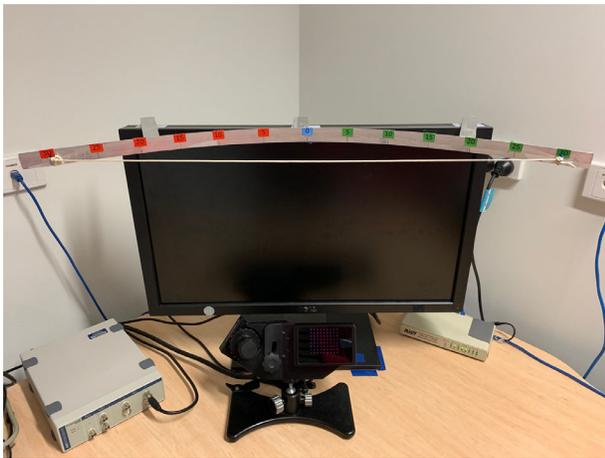
FIGURE 1. A metal arc mounted to the top edge of the monitor with targets at  $\pm 30$  degrees from the center in 5-degree steps. It was used to measure the gaze position of the subject.
