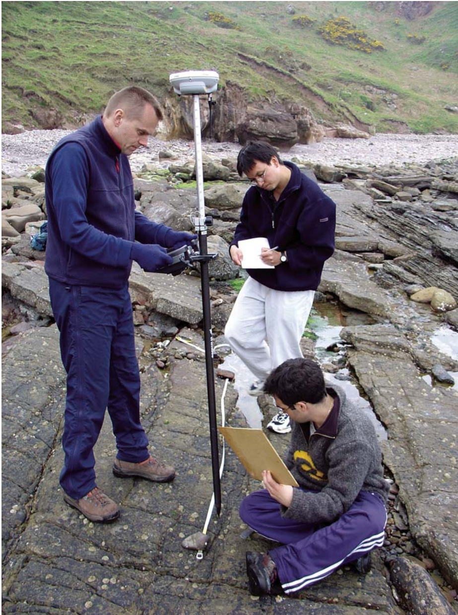
← Figure 1. Comparison of traditional and digital line sampling (line samples are generally considered to be one-dimensional [1D] data sets). Traditional line sampling (geologist on right) takes measurements at recorded distances along the tape measure; the dimensionality of the data set (1D) matches the single coordinate axis used to record each measurement (i.e., length along the tape). In contrast, using differential global positioning system (GPS) (geologist on left), each measurement along the line records the precise X, Y, and Z position of that point; hence there is a mismatch between the dimensionality of the data set (1D) and the dimensionality of the coordinate system used to record the measurements (3D). (From a study analyzing variation in throw along the length of fault traces, Lambertton, southeastern Scotland, in which resolution and precision of traditional and digital methods were compared. Photo courtesy Phill Clegg.)
