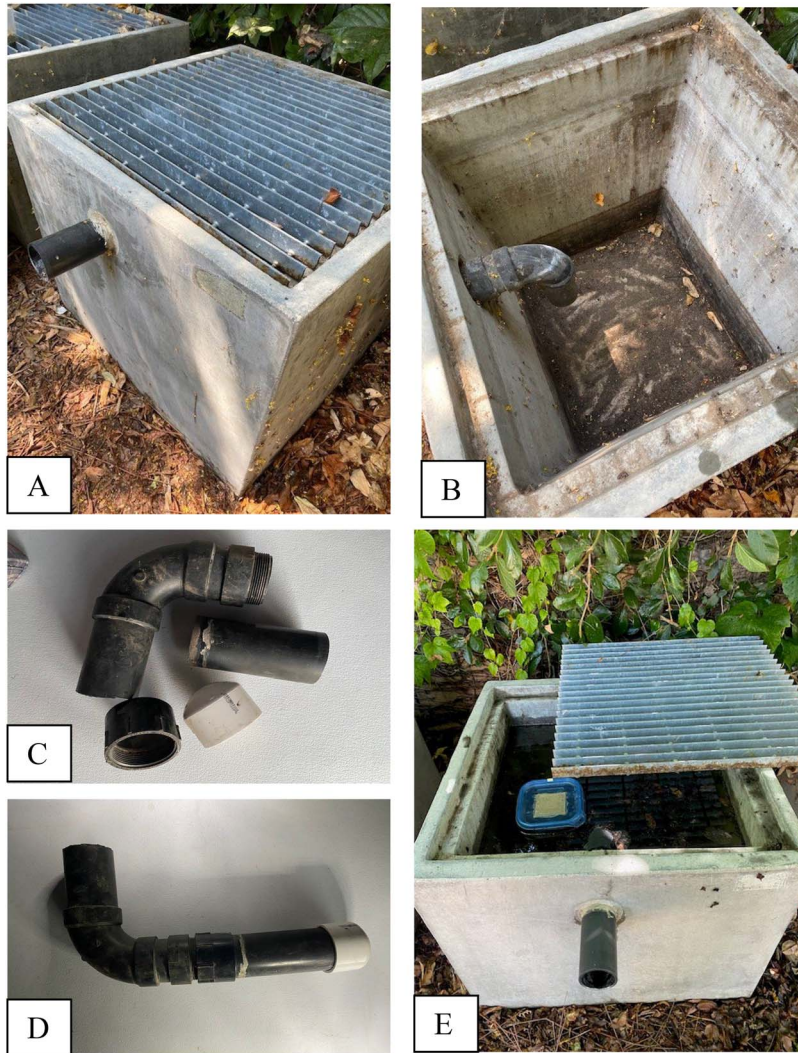
Fig. 2. Cast concrete simulated catch basin: exterior overview (A), interior overview (B), drainpipe components (C), assembled drainpipe (D), and basin in operation (E).
