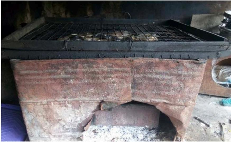
Figure 1 — An open-drum traditional kiln
