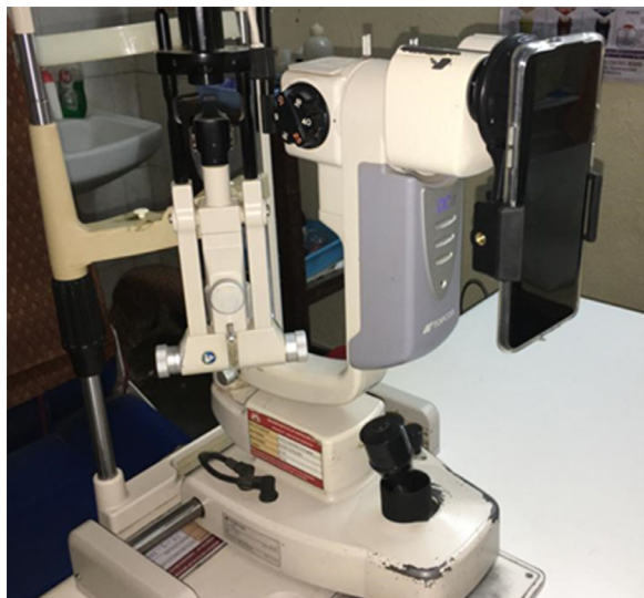
Figure 1. Imaging setup of smartphone-based method. OnePlus 7 Pro smartphone is shown attached to the Topcon slit lamp.
