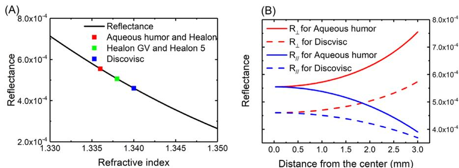
**Figure 2.** (A) Reflectance at normal incidence according to the refractive indices of various ophthalmic viscosurgical devices. (B) Reflectance of perpendicular ( $R_{\perp}$ ) and parallel ( $R_{\parallel}$ ) to the incident plane of laser, according to the various incident angles for aqueous humor and Discovisc.
