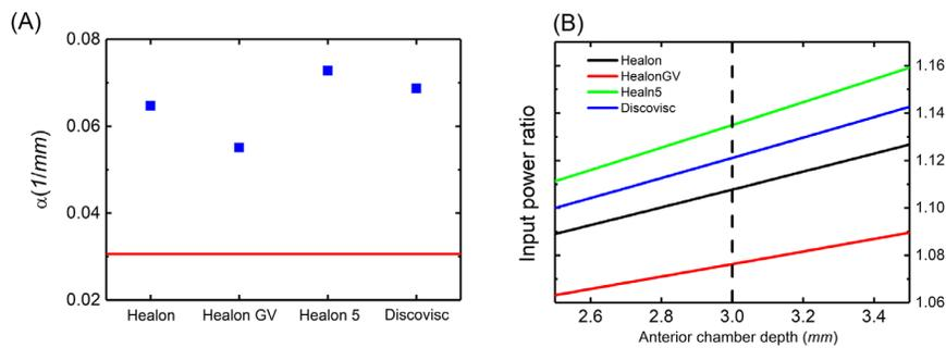
**Figure 4.** (A) Measured absorption coefficients of various ophthalmic viscosurgical devices and the water (red line). (B) Input laser power ratio to achieve the same power intensity as aqueous humor.
