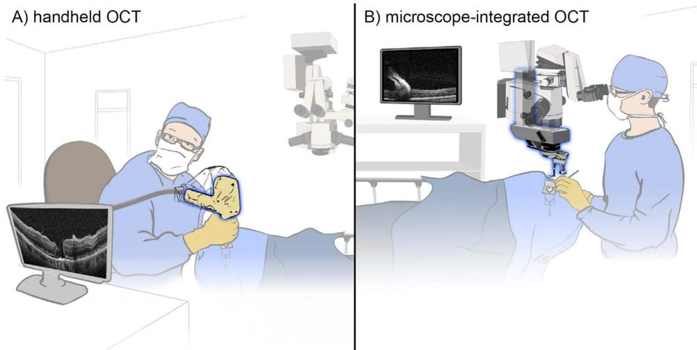
**Figure 1.** Illustration comparing the use of HHOCT and MIOCT. HHOCT (A) requires a full pause in surgery, removal of the microscope away from the surgical field, and placement of a portable OCT scanner with a sterile wrap over the eye to obtain images viewed on a separate computer screen. In contrast, MIOCT (B) is integrated into the surgical microscope, enabling OCT acquisition simultaneous with ongoing surgical manipulations. Instrument-retina interactions can only be imaged with MIOCT.
