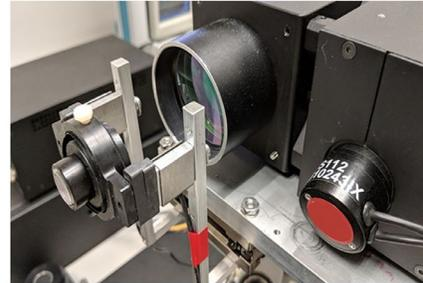
**Figure 1.** Left: schematic representation of the optical coherence elastography system. Right: picture of the prototype, with a focus on the transparent flat lens, force sensors, and translational stage. SS-OCT, swept-source optical coherence tomography system.
