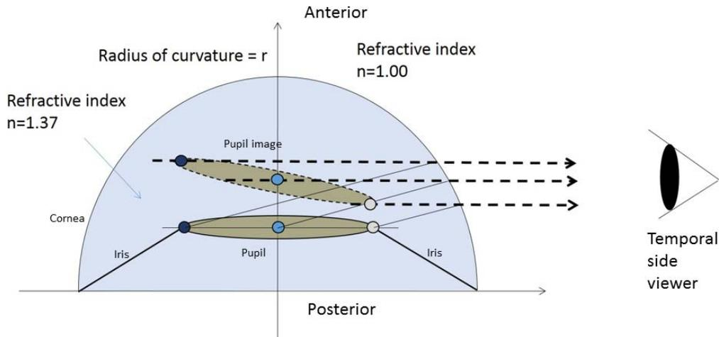
**Figure 5.** Corneal-Aqueous refraction results in the formation of a virtual, oblique pupil image anteriorly to the true pupil plane. The further the object is from the viewer, the more anteriorly is its image displaced.
