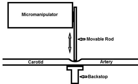
**Figure 1.** Schematic diagram of apparatus for graded compression of the CA in rats. The micromanipulator allows for precise positioning of the movable rod in the directions indicated by the *double-headed arrow*. This permits controllable compression of the CA between the movable rod and backstop.
