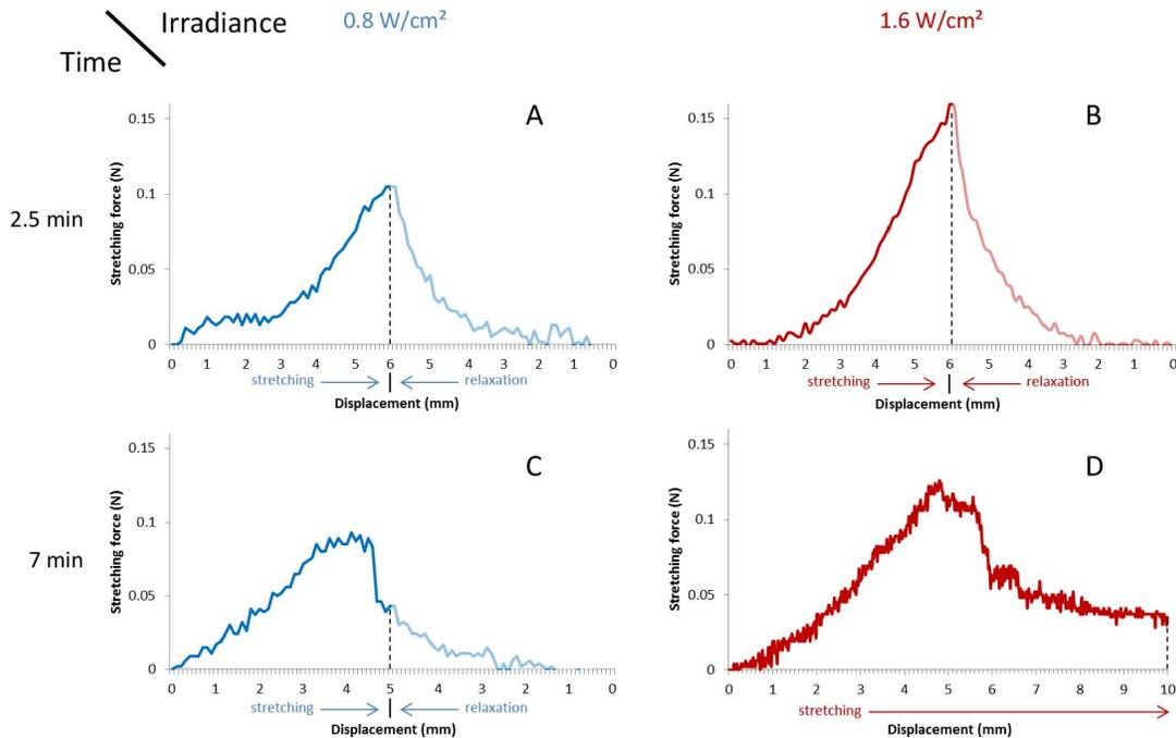
**Figure 4.** Stretching–relaxation cycles of the photobonded samples irradiated with different irradiances and times. The Figure shows the last stretching cycle of each sample. Samples A and B have symmetric and continuous response around the maximum force, coincident with the maximum displacement. In samples C and D, there is an abrupt force decrease that occurs before the maximum stretching distance, consistent with a tissue breakage. See text for details.
