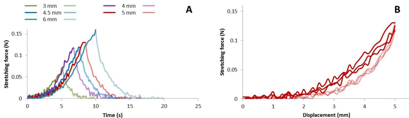
**Figure 3.** (A) 3, 4, 4.5, 5, and 6 mm stretching cycles of the photobonded sample irradiated at  $1.6 \text{ W/cm}^2$  for 2.5 minutes. *Dark line* corresponds to the stretching period and the *light line* corresponds to the relaxation period of the cycle. (B) 5 mm stretching–relaxation cycle (three consecutive repetitions).
