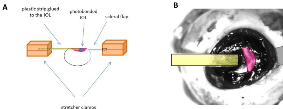
**Figure 2.** (A) Set up of the stretcher with the sample mounted. (B) Photograph of the plastic strip (yellow) glued to the photobonded IOL (pink). The scleral flap (gray) and plastic strip are clamped to the stretcher.
