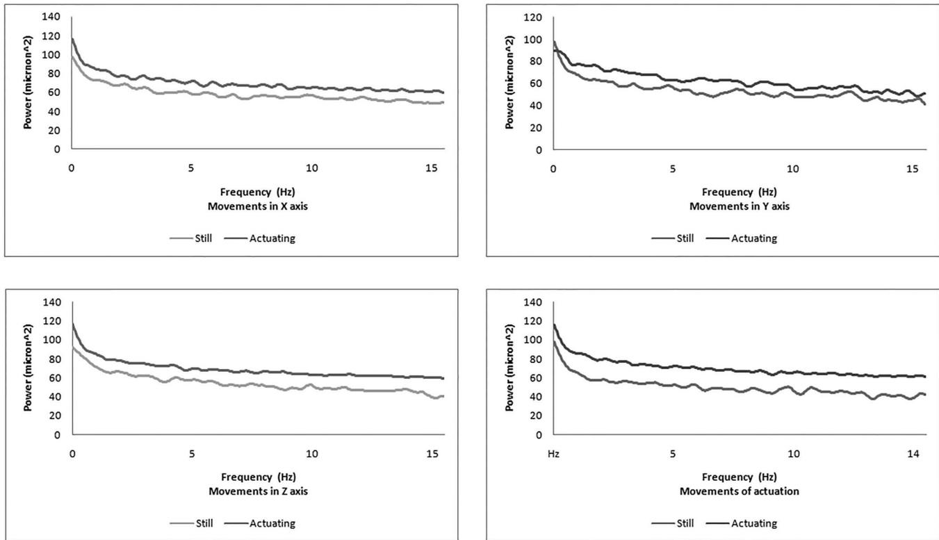
**Figure 2.** Averaged Fourier frequency analysis of the movements in  $x$ ,  $y$ , and  $z$  axes and also of the actuator, referred to as the  $a$  axis recorded during actuation and holding the instrument motionless. Note there is an area of higher amplitude with narrow peaks at  $<5$  Hz and areas of lower amplitudes with broader peaks at 7 to 13 Hz.
