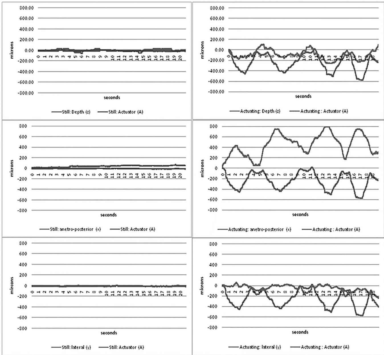
**Figure 3.** Sample recordings from an individual attempt. The *left column* represents the unintentional movements during actuation and the *right column* represents the subject attempting to hold the instrument motionless. The large actuation artefact is clearly visible in the curves in the left column.
