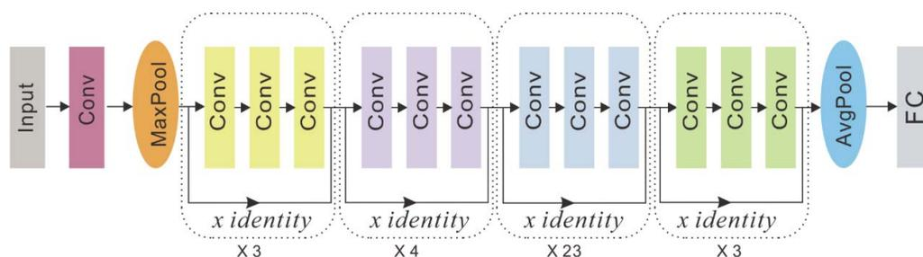
**Figure 3.** A diagram showing a 101-layer ResNet. Conv, convolutional layer; AvgPool, average pool; FC, fully connected layer.
