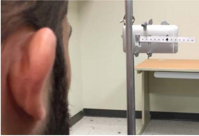
Figure 3. Experimental setup to measure the accuracy of the app in Study 1. Subjects without strabismus fixated on 13 targets on the rear side of a smartphone placed at a distance of 30 cm with their head resting on a chin-head rest. Twelve of the 13 fixation targets were a black cross on a white background. The center target was the smartphone camera. With the known distances, true eye deviation magnitudes with respect to the central fixation point were computed (angular range covered by the fixation targets was \pm 13^\circ or \pm 23\Delta ) and compared to measurements with the app.
