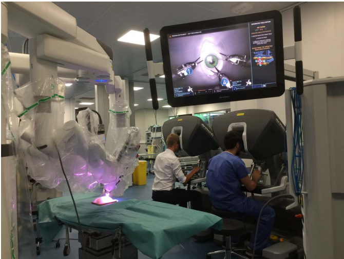
Figure 1. Installation. On the left side are the surgical tables with the strabismus dry-lab training system installed under the robotic da Vinci Xi Surgical System above it. On the right side and in the background are the surgeon's remote consoles. The video screen ( top ) shows the operative field with the three robotic arms above the eye model.
