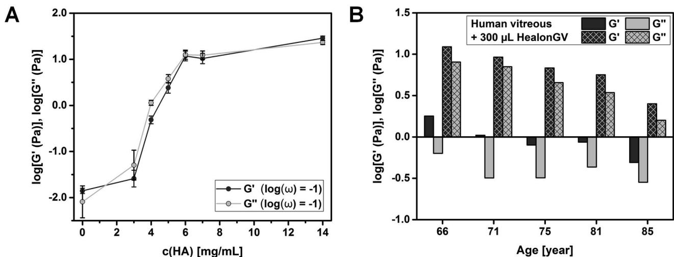
**Figure 4.** (A) Increased dynamic moduli of HA solutions with increasing HA concentration and gel-like behavior (storage modulus  $G' >$  loss modulus  $G''$ ) at 14 mg HA/mL (Healon GV). The *error bars* display the standard deviations of three independent experiments. (B) Low viscoelastic properties of human vitreous bodies extracted from old donors were enhanced due to the intravitreal injection of 300  $\mu$ L Healon GV.
