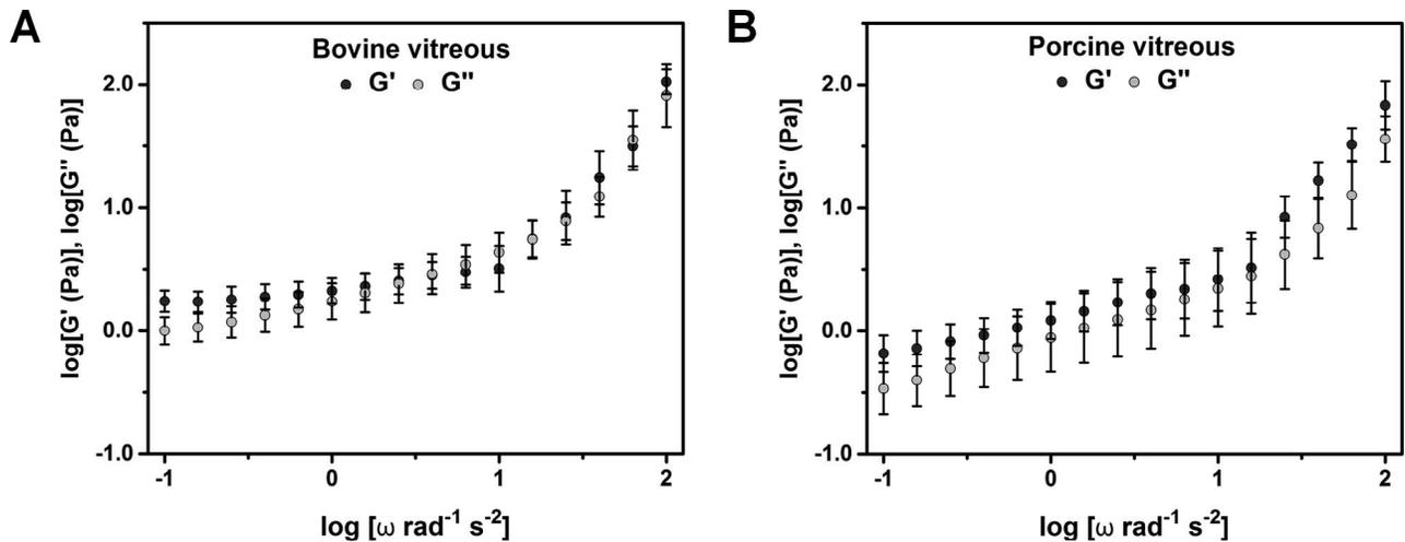
**Figure 3.** Frequency sweep tests of extracted bovine ( $n = 15$ ) (A) and porcine ( $n = 15$ ) (B) vitreous bodies. The *error bars* display the standard deviations. Storage moduli  $G'$  were found to be higher than loss moduli  $G''$  at low frequencies indicating a gel-like behavior for both animal sources (with bovine  $>$  porcine,  $P < 0.001$ ).
