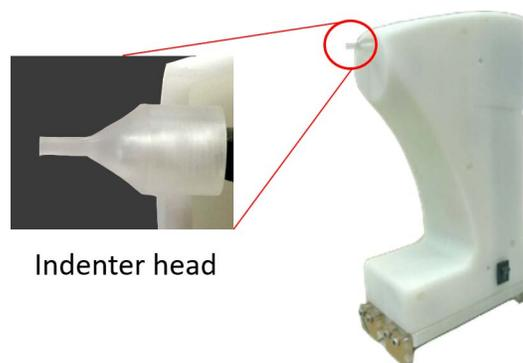
**Figure 3.** Corneal indentation device and corneal indenter (US Patent WO2012163080 A, 2012).
