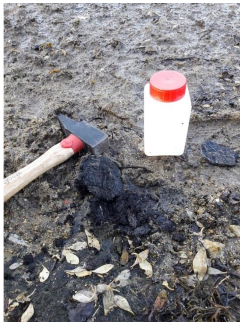
Figure 3. Asphalt pavement buried in salt marsh (Sample #AM2).
