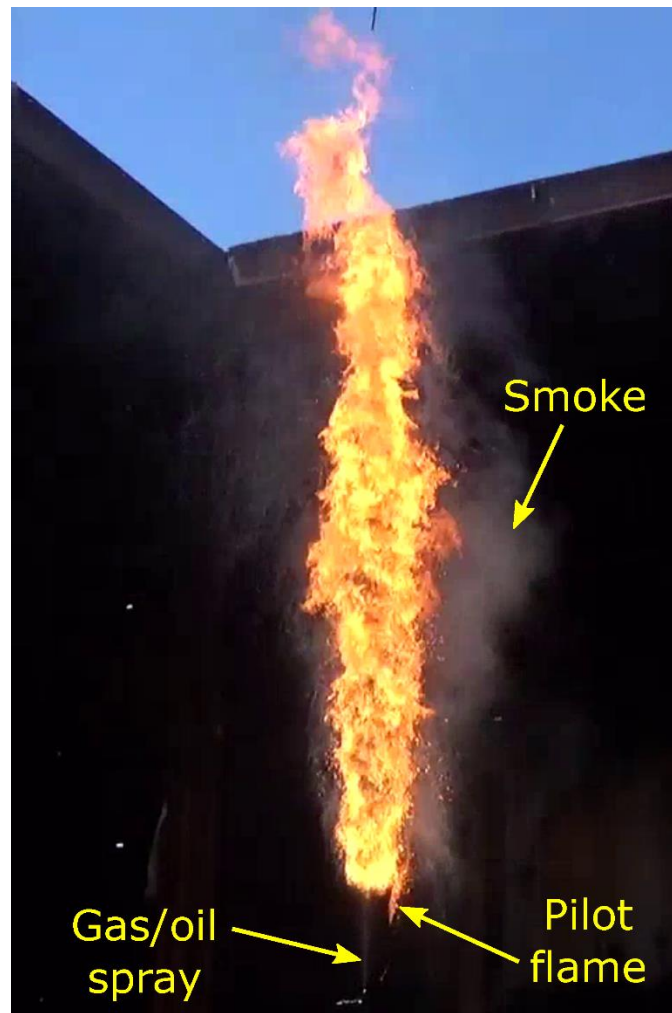
Figure 4. Gas/oil spray flame image, viewed from SE corner of test chamber.
