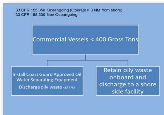
Figure 2: Flow Chart Display for Code of Federal Regulation Requirement's for All Commercial Vessels
