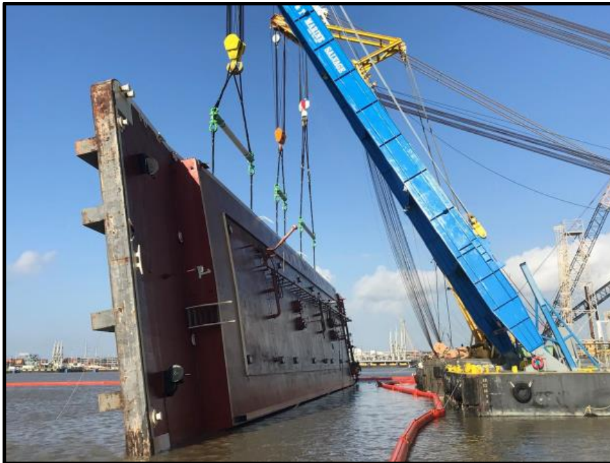
Tank Barge Lightering and Parbuckling Operations in Houston Ship Channel (T&T Salvage)
