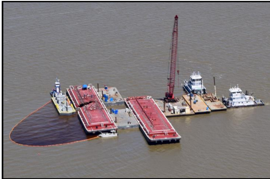
Tank Barge Lightering Operation in Houston Ship Channel (T&T Salvage)
