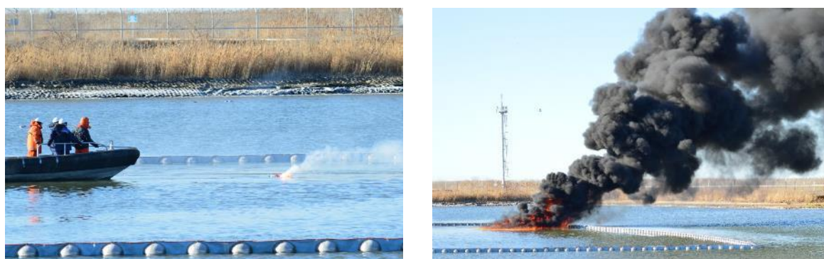
Figure 10. Oil ignition and burn
