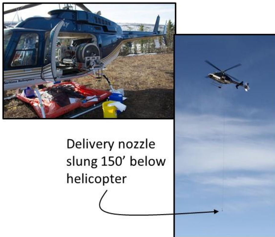
Figure 2. Photos of the prototype helicopter herder delivery system in the cabin of a helicopter (left image) and deploying the 150' hose and nozzle assembly during flight.
