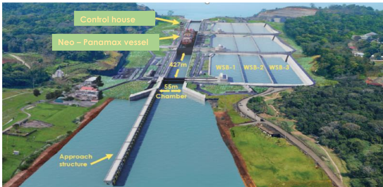
Figure 2. Panamá Canal expansion project illustration. (Credit: ACP)
