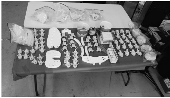
Figure 1 - An array of cast and manufactured parts ready for assembly. This represents enough parts for 4 mannequins.
