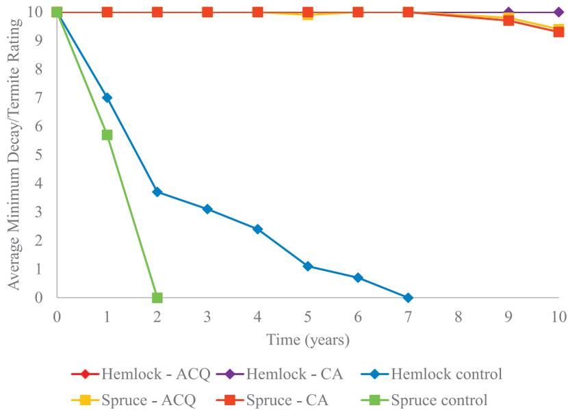
Figure 6.—Average lowest (decay/termite) ratings of white spruce and western hemlock stakes untreated or treated with ACQ or CA-B in a ground contact stake test in Jinju, Korea. ACQ = alkaline copper quaternary; CA-B = copper azole, Type B.
