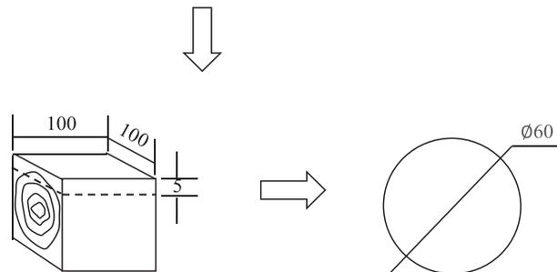
c. Cutting 5-mm-thick surface layer from the surface of 100-mm-long section
