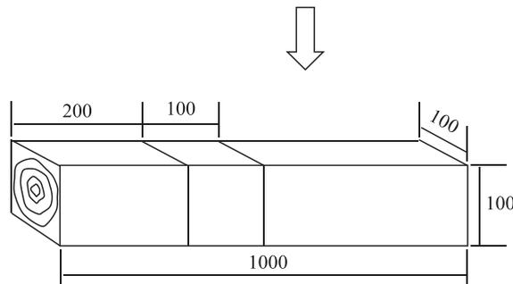
b. Cutting 100-mm-long section from drying
