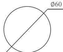
d. Cutting rounded specimen from 5-mm-thick layer
